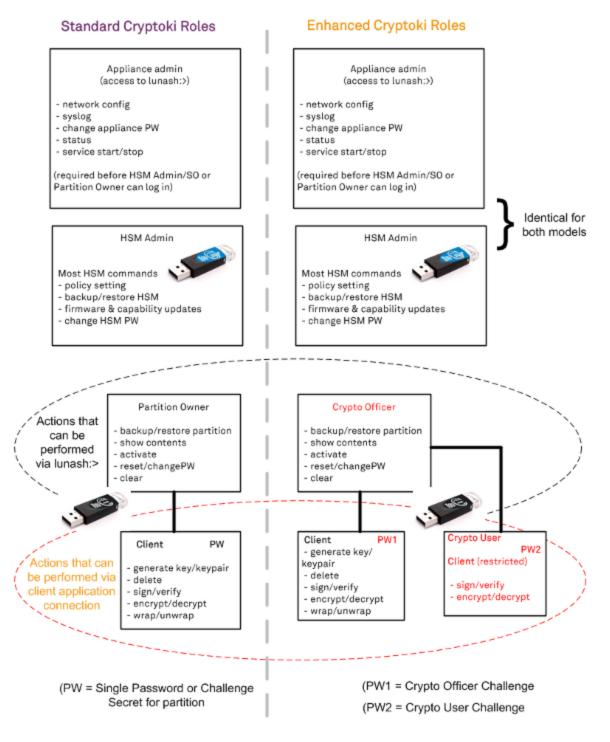
The Crypto Officer and Crypto User roles, described on the right-hand side of the diagram (above) exist only for Luna HSM with Trusted Path Authentication. They don't exist for a Luna HSM with Password Authentication.
