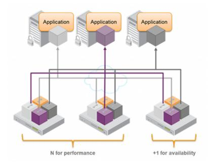
As performance needs grow beyond the performance capacity of three HSMs, it often makes sense to define a second independent group of application servers and HSMs to further isolate applications from any single point of failure. This has the added advantage of facilitating the distribution of HSM and application sets in different data centers.
